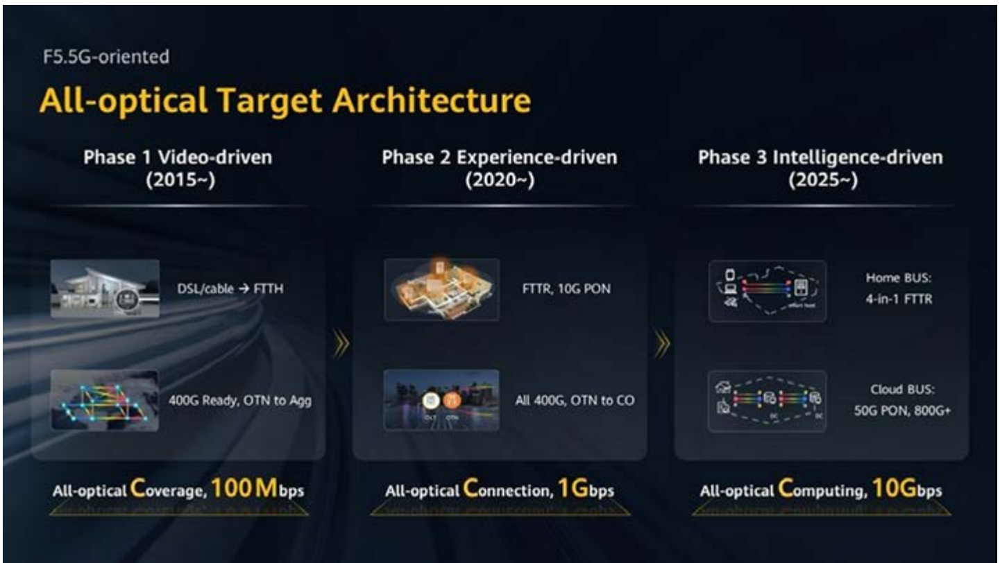
F5.5G-oriented three-phase all-optical target network architecture
